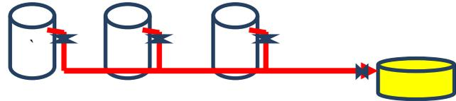
Usually everything went well, but on occasions there would be severe hammering in the line as discharge started. Usually this was no more than worrying and required no more than restoring pipes to their proper location. Occasionally things were worse, but the standard fixes (altering valve stroking rates etc.) did not seem to help.
