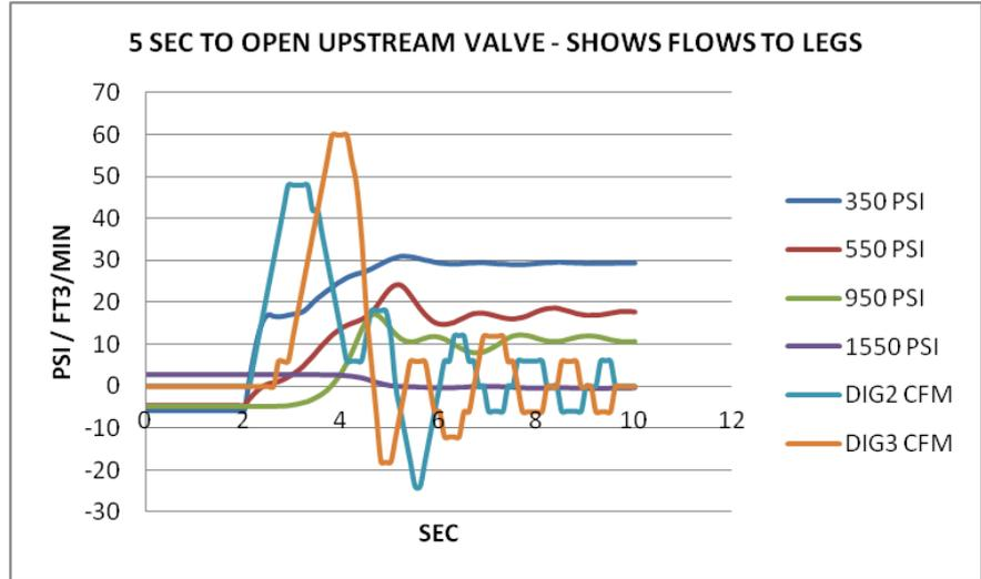
The problem could have been fixed by re-running the horizontal pipe at a higher level to eliminate the drop legs. However, in this case it was easier to place non-return valves at the bottom of each leg. This converted the unstable flow shown above to the very stable flow shown below:
