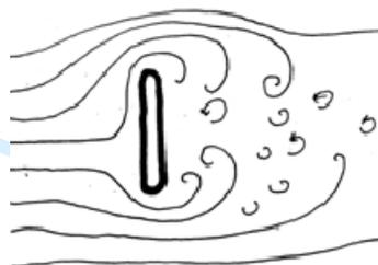
stopping the air flow; destroying all of the kinetic energy.
