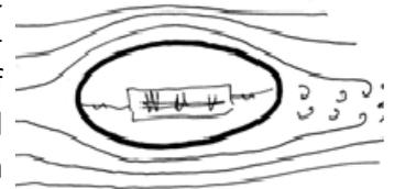
(which is pretty "streamlined") the wake is probably about 30% of the frontal area. So your hand would be said to have a "drag co-efficient ( $C_d$ )" of 1.2 and the football around 0.3. The losses all relate directly to the kinetic energy, and hence the velocity pressure. That's how it works.
